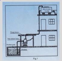
The figure represents the installation of the pump within lightning weight, no special foundation is needed. Just Place the pump on the ground level over a base, or you can hang inside the well.
